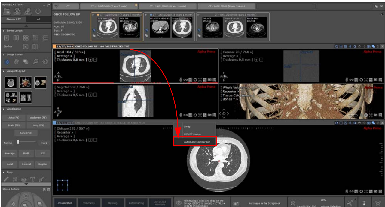
Figure 13-15 Automatic opening of the desired series in the 'Automatic Comparison' protocol using drag & drop
