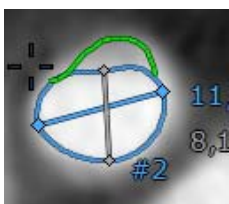
Figure 11-128 Example of manual modification of a cross-section contour using the 'Alt' key and the left mouse button
